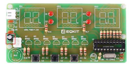
Step 14:Install 1pcs 10uF/25V Electrolytic Capacitor at C1.Pay attention to the installation direction and the shorter pin is negative pins.
